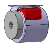
7- Draw the filter/filter support assembly close to the LHS of the motor and apply the filter by exerting pressure and making sure the filter slot coincides with the projection on the motor as shown in the figure.
