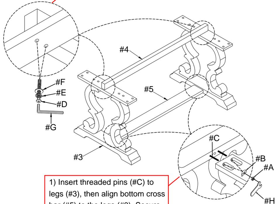
1) Insert threaded pins (#C) to legs (#3), then align bottom cross bar (#5) to the legs (#3). Secure by using washers (#B) and hex nut (#A).
