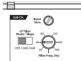
**2) LP Filter Operation:** The low-pass filter in the M1000/1v2 is fully variable between 50 Hz and 500 Hz via the “**Filter Freq.**” control knob and features the ability to select between a moderate “**12dB**” per octave or a steep “**24dB**” per octave slope via the “**LP Filter Mode/Slope**” switch.
