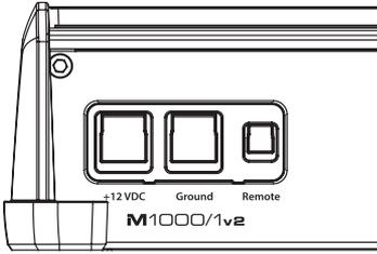
The M1000/1v2's “+12 VDC” and “Ground” connections are designed to accept 4 AWG power wire. **4 AWG is the required wire size for this amplifier.**
