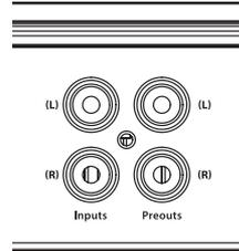
You may run a stereo or a mono signal into the inputs of the amplifier. The amplifier's input section automatically sums stereo signals to mono for the internal amplifier section. The amplifier will operate with only one input connection (left or right), but will require an increase in input sensitivity to overcome the loss of signal. If a mono input signal is to be run, we recommend that you use a “Y-adaptor” to split the mono signal into both inputs of the amplifier.
