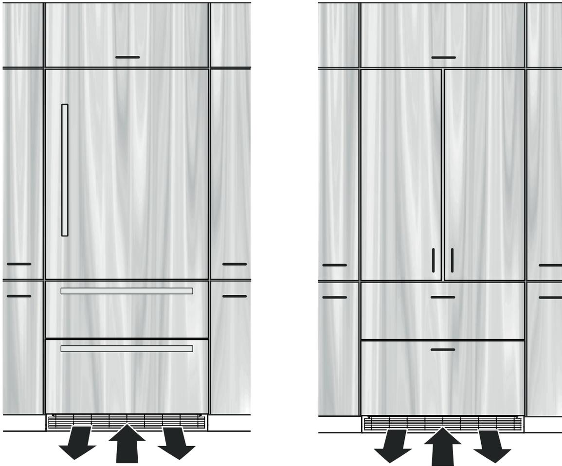
It is important to use the provided cover grille for the ventilation opening. This opening must not be covered.
