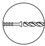
2. Match the drill bit to the wall anchor and hole size.
