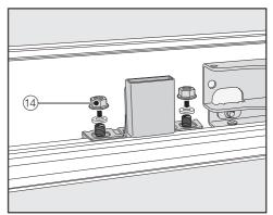
Place the washers and nuts <sup>(1)</sup> back in position and tighten the nuts <sup>(1)</sup>. The appliance door is now fixed.
