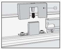
■ Fit the cover ② to the light contact switch.
