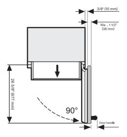
\* The dimensions of the cabinet front and the door handle vary depending on the design of the kitchen.
