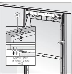
Screw the lugs for the fixing plate (10) into the cabinets/units above the wine conditioning unit. If it is not possible to secure the wine conditioning unit at the top, it can be attached to the niche with the side fixing plates:
