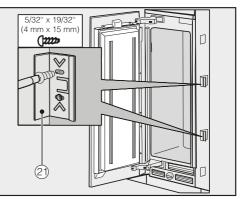
Secure both sides of the wine conditioning unit using at least 3 clips for the covers.
