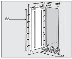
Fit the two plastic covers <sup>(20)</sup> on both sides of the appliance door by clicking them into the gap between the appliance door and the cabinet door, starting at the bottom and working up to the top.
