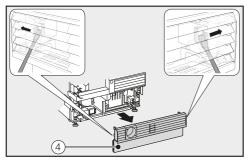
Carefully guide a flat-head screwdriver through the grate in the baseboard ④ on both sides and use it to push the internal plastic latches outwards to release the baseboard.
