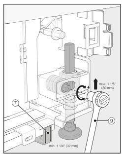
Adjust the front feet with a ratchet (attachment: 5/16" (8 mm)) socket) or a TX 20 screwdriver (9).
