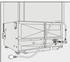
Insert the plug into the back of the wine conditioning unit.
