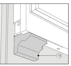
Click the cover <sup>(B)</sup> onto the fixing bracket.
