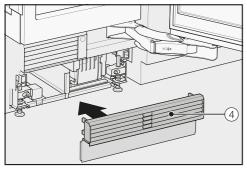
Click the toe-kick ④ onto the bottom of the base of the wine conditioning unit.
