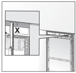
Measure the gap X between the adjusting bar and the upper edge of the adjacent cabinet front.
