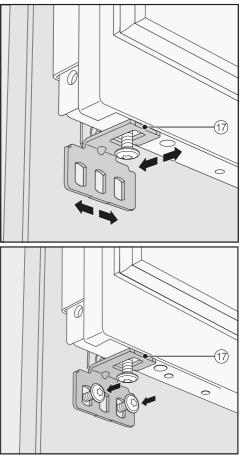
Screw the fixing bracket securely to the cabinet front.
