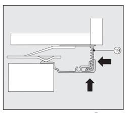
Place the assembled cover <sup>(1)</sup> into the gap above the wine conditioning unit so it clicks into place. While doing so, slide both parts of the cover together as required.
