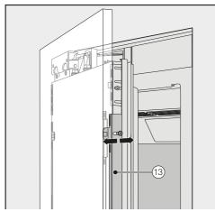
Align the depth of the appliance door via the gaps in the angle trims <sup>(1)</sup>3. Then screw the angle trims <sup>(1)</sup>3 into position.
