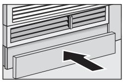
Do not cover the vents in the base. This will damage the wine conditioning unit!
