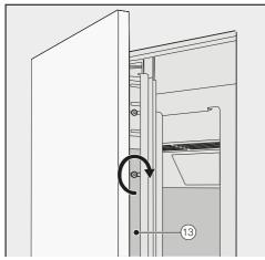
■ Now tighten the screws in the angle trims <sup>(3)</sup>.
