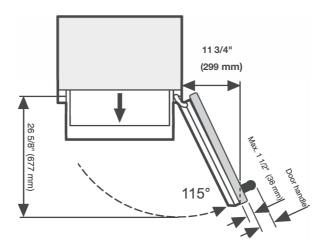
\* The dimensions of the cabinet front and the door handle vary depending on the design of the kitchen.
