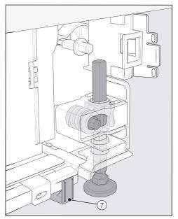
Position the supplied spacers ⑦ on both sides on the markings next to the adjustable feet at the front of the wine conditioning unit.
