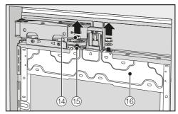
Remove the nuts and washers <sup>(1)</sup> from the threaded bolts <sup>(1)</sup>s and store them in a safe place – they will be required later.
