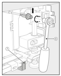
Adjust the rear feet with a ratchet (attachment: 5/16" (8 mm) socket) or a TX 20 screwdriver (8).
