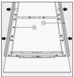
Now insert the angle trims <sup>(1)</sup> as far as they will go into the provided spaces in the fixing frame <sup>(1)</sup>.
