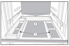
Next, place the accessory boxes ① on either side of the shelf (the large box to the left) and position the decanter plate ② in the center of the shelf.
