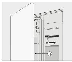
Unscrew the angle trims (3) from the appliance door and place the trims and screws to one side – they will be required later.
