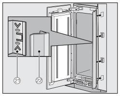
Now attach the covers 2 onto the retaining clips 1 on both sides. In the case of side-by-side installation, the covers are only required on the outer side.
