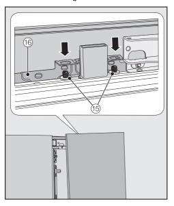
Open the door of the wine conditioning unit and hang the cabinet front on its frame (16) onto the threaded bolts (15).
