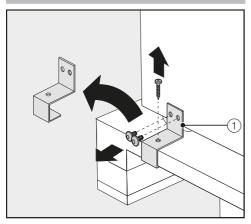
Unscrew the brackets (2) that are fixing the wine conditioning unit to the delivery pallet. With the help of several people as required, carefully lift the wine conditioning unit from the pallet, starting with the back of the wine conditioning unit.
