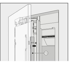
Press the angle trims (13) into the white plastic frame on both sides and screw them securely into place. Spare screws are provided in the plastic bag marked with the letter E.
