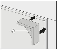
Place the spacers ⑦ on top of the cabinet front on both sides.
