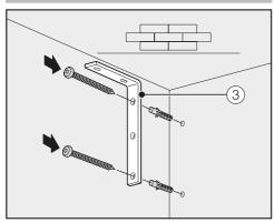
Securing to a concrete wall
