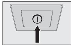
Turn the wine conditioning unit on by pressing the On/Off switch.
