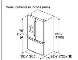
A: Add 5/8" (17) with front leveling feet fully extended
