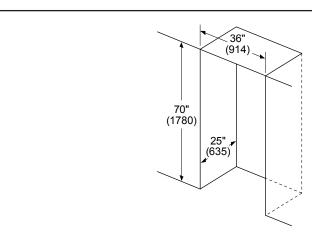
Leave 1/2" (12.7) gap at the top and 1" (25.4) behind the refrigerator for proper ventilation.
