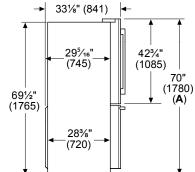
A: Add 5/8" (17) with front leveling feet fully extended
