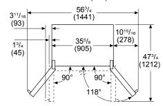
Drawers can be pulled out with door open to  $90^{\circ}$ Drawers can be taken out with door completely opened
