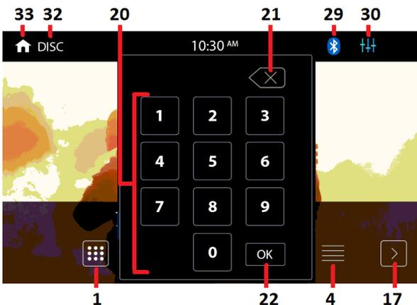
1. Touch to activate **KEYBOARD INTERFACE** to input track number directly for playback.
