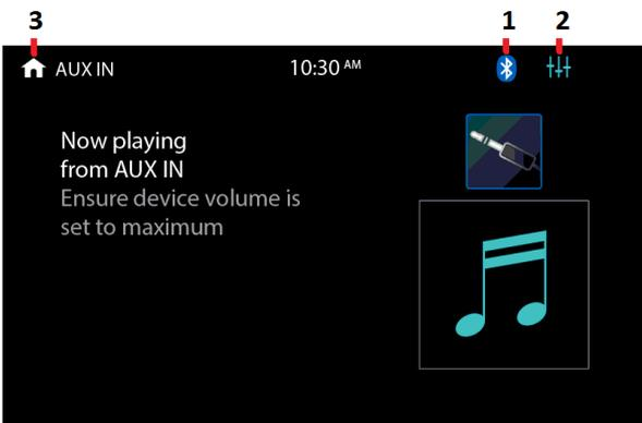
1. This Bluetooth icon will light up if the unit has connected to a mobile phone. If no connection made, the icon will flash.
