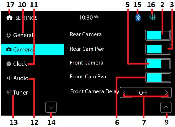
1. Touch repeatedly to select the front or rear camera viewing when the car is shifted from forward mode to backward mode. When "Off" is selected, no camera viewing available at car backward mode.
