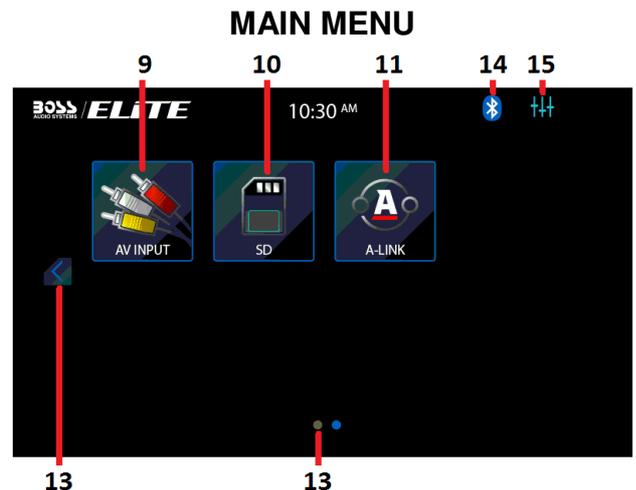
At **MAIN MENU**, touch the icon of the desired mode on screen and the unit will then enter into the mode that selected for operation.
