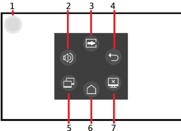
1. Touch to activate **FLOATING DOCK MENU** on screen for various functions and controls of the unit. Hold & slide can move this icon to other desired position on the screen.
