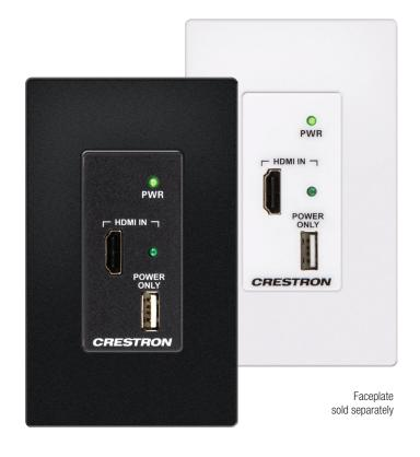
The HD-TX-101-C-1G-E series comes in black or white, and is designed to mount in a single-gang electrical box or plaster ring (not included). It is normally powered by the receiver over the link cable when using a surface mount receiver. If using a wall plate receiver, a single power pack must be purchased (sold separately, model TBA), which may be connected to either the transmitter or receiver. [2]
