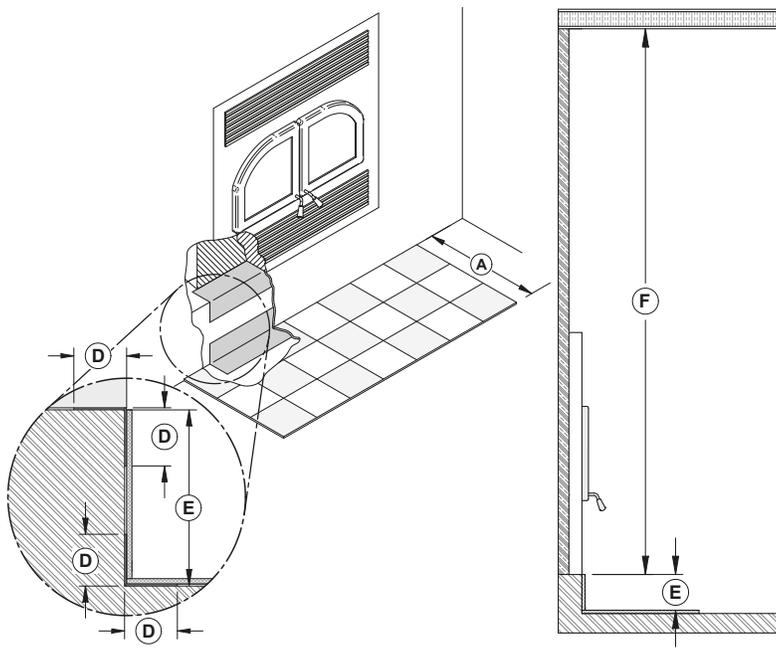
When the fireplace is installed on a raised base of more than 4" (E), a non-combustible floor protection of at least 16" (A) with no R factor must be installed in front of the fireplace.
