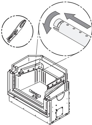
2. Align the notch in the left end of the tube with the key of the left air channel hole. Using a «Wise grip» hold the tube and lock it in place by turning the tube as shown. Make sure the notch reaches the end of the key way.
