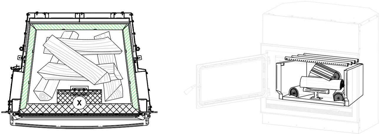
The images above show the space in the firebox where the logs are to be placed. It is important to always respect this space and not to put logs in the grid area marked with an X. The marked area is defined by the space between the glass and the cast-iron andiron. To have a good ignition, place the two lower logs in a north-south position and cross the others on top. Leave enough space between the logs for good air circulation. The log length recommended for this fireplace is 16 in.
