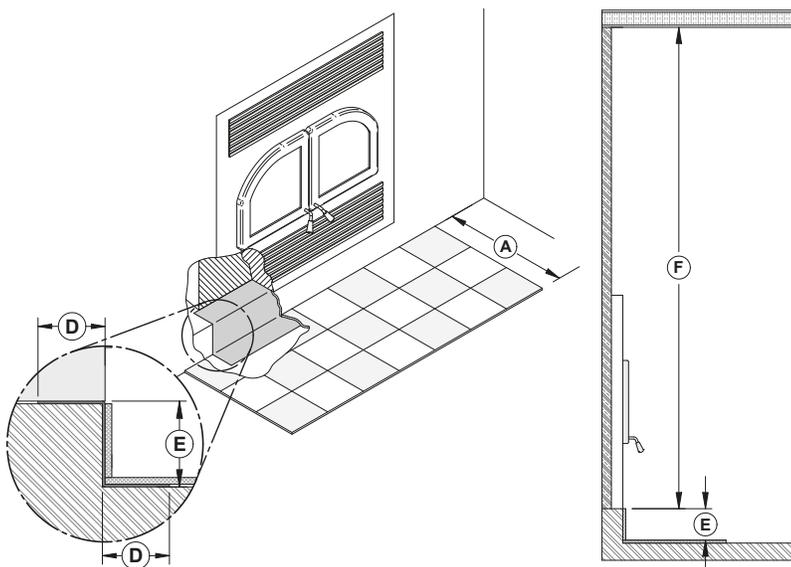
When the fireplace is installed on a raised base of 4" or less **(E)**, a non-combustible floor protection of at least 16" **(A)** with an R factor of 1.00 must be installed in front of the fireplace.
