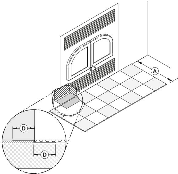
When the fireplace is installed directly on the floor, a non-combustible floor protection of at least 16" **(A)** with an R factor of 1.00 must be installed in front of the fireplace.
