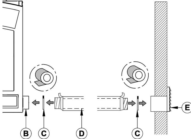
5. To complete the installation, make a hole of  $\frac{1}{4}$ " to  $\frac{1}{2}$ " (6 mm to 13 mm) bigger than the duct diameter on the outside wall of the house at the chosen location. From outside, place the outside wall register in the hole (open side down) and fasten the register to the wall, with screws.
