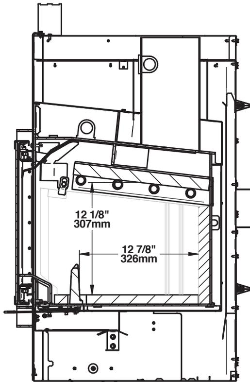
Combustion chamber - Side view
