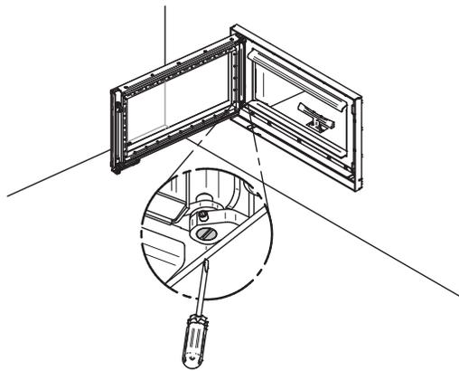
Using a flat screwdriver, turn the adjustable hinge rods in the directions shown to adjust the doors. Tighten the set screws on the door hinges when they are in the desired positions.
