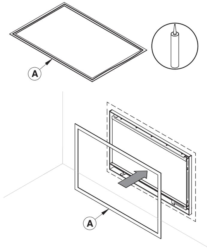
Secure the finishing frame to the facing using silicone.
