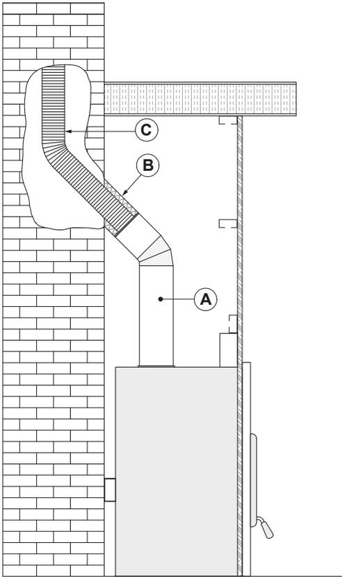
1. Position the fireplace in its location. Temporarily install the elbow or chimney section **(A)** on the top of the fireplace and, using a level, mark with an oval the location where the flue liner will enter the masonry chimney.
