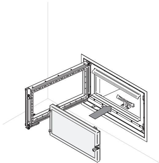
3. Lean the upper part of the firescreen against the top door opening making sure to insert the top firescreen bracket behind the primary air deflector.
