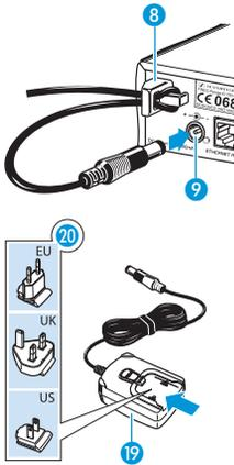
Only use the supplied mains unit. It is designed for the transmitter and ensures safe operation.
