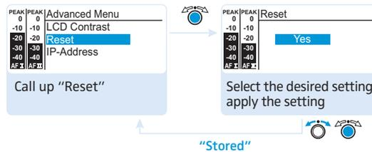
When resetting the settings made in the operating menu, only the selected settings for the pilot tone and for the frequency banks “U1” to “U6” remain unchanged. For an overview of the factory-preset default settings, refer to the enclosed frequency information sheet.
