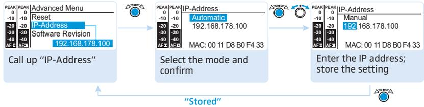
You can either automatically allocate or manually enter an IP address. This menu item also shows the transmitter’s unique and unchangeable MAC address. In order to ensure safe communication between transmitters in multi-channel systems (see page 33), we recommend using automatic allocation of IP addresses.
