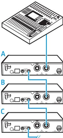
To daisy chain an audio signal from one transmitter to the next:
