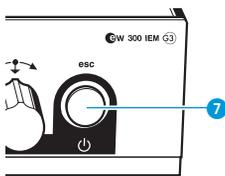
To switch the transmitter to **standby mode**:
