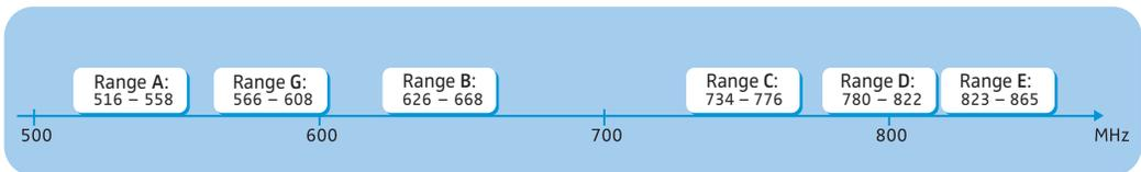
Each frequency range (A–E, G) offers 26 frequency banks with up to 16 channels each:
