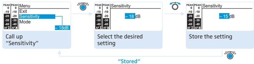
Adjustment range: 0 to -48 dB, adjustable in steps of 3 dB
