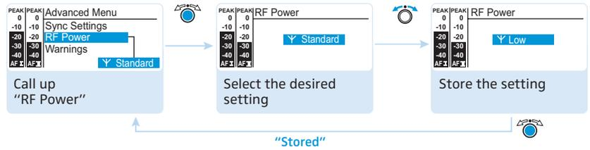
Via the “RF Power” menu item, you can adjust the transmission power in two steps (Low, Standard).
