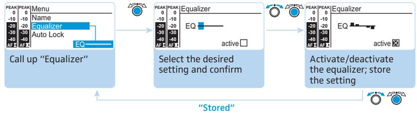
Adjustment range:  $\pm 12$  dB, adjustable in steps of 2.4 dB
