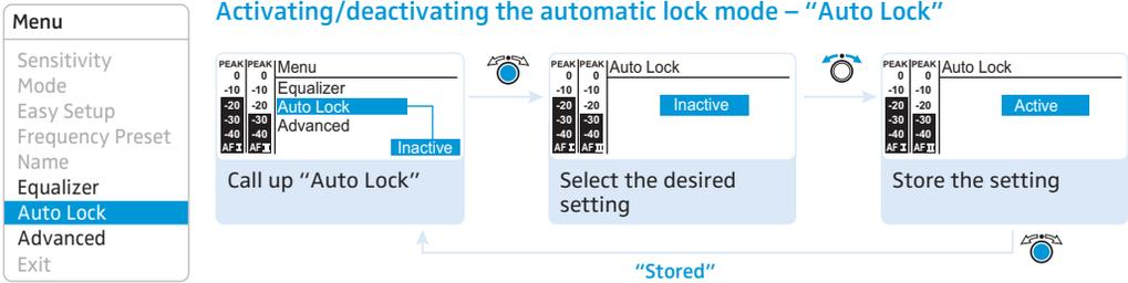
The lock mode prevents that the transmitter is accidentally switched off or programmed during operation. The lock mode icon
