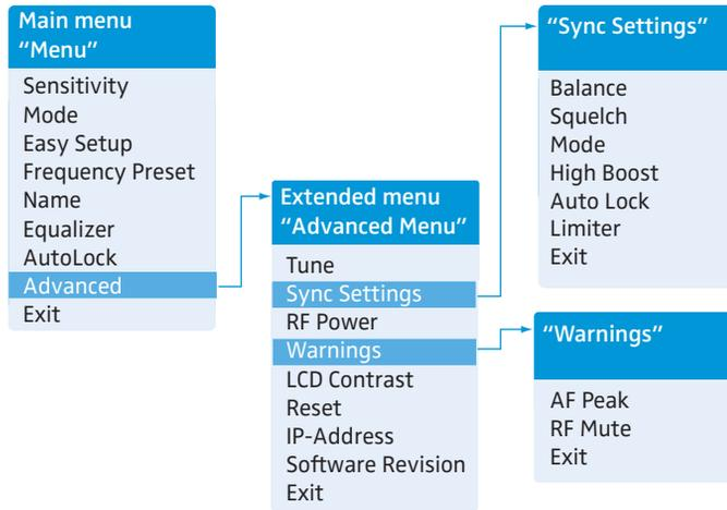
When the standard display is shown on the display panel, you can get into the main menu by pressing the jog dial. The extended menu “Advanced Menu” and the other menus can be accessed via the corresponding menu items.
