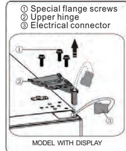
4. Remove the upper door from the middle hinge by carefully lifting the door straight up. Then place the upper door on a smooth surface with its upper cover upwards.
