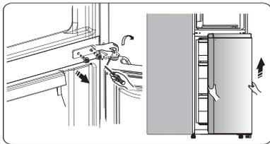
9. Place the lower door on a smooth surface with its panel upwards. Loose screw ③ and take down part ② and part ①, install replacement door stopper-left ④ provided (in the plastic bag) and part ②(stop block) to the left side with screw ③. Keep part ① with the appliance for future reference.
