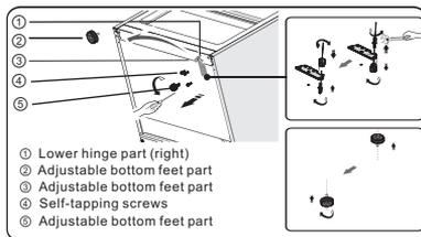
12. Remove part ③ from the lower hinge pin, loose out the lower hinge pin, change it to the reverse hole site, and then tighten into position, then install part ③ on the lower hinge pin.
