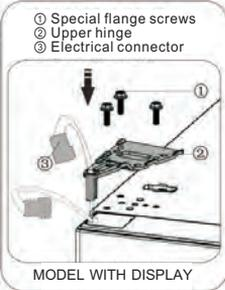
16. Connect electrical connector ① as shown in the picture, then fix part ② by screw ③ refer to step 2.
