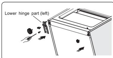
14. Slot the lower door onto the bottom hinge pin and hold in position. Turn the middle hinge by 180°, change the washer on the axis to the lower side, adjust the middle hinge to the appropriate position and then install it ensuring the lower door in secured place.
