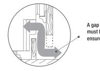
A gap of 1 3/8" (35 mm) must be maintained to ensure sufficient ventilation.
