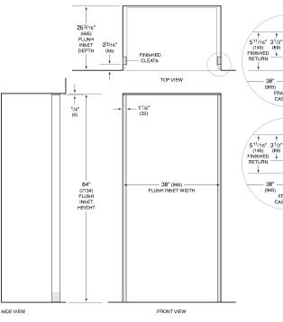
NOTE:  $3^{1/2^{\prime\prime}}$  (89) finished returns and shaded areas will be visible and should be finished to match cabinetry Shaded line represents profile of unit with  $3^{1/4^{\prime\prime}}$  (19) panel.
