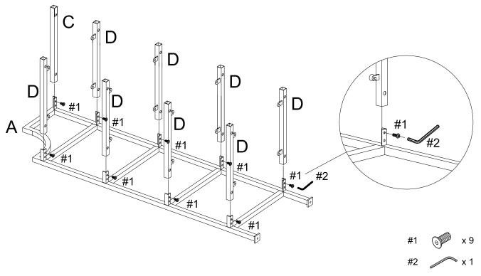
Step 2. Attach right frame (part B) into cross rail (part C) and shelf rails (part D) using bolts (part #1) and allen wrench (part #2).
