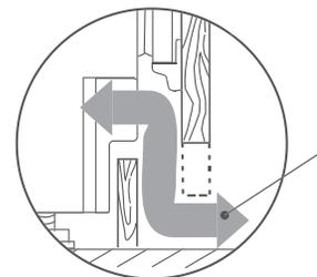
**A gap of 1 3/8" (35 mm) must be maintained to ensure sufficient ventilation.**
