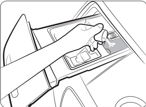
Add only liquid chlorine bleach to the **bleach compartment**. Do not exceed the **max line**.
