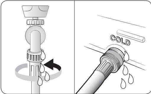
5. Connect the other ends of the water hoses to the corresponding inlets on the rear of the machine as specified. Make sure the hot water hose is connected to the hot inlet, and the cold water hose to the cold inlet.
