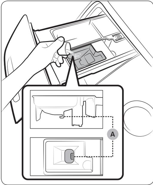
3. Add fabric softener to the **softener compartment**. Do not exceed the **max line (A)**.
