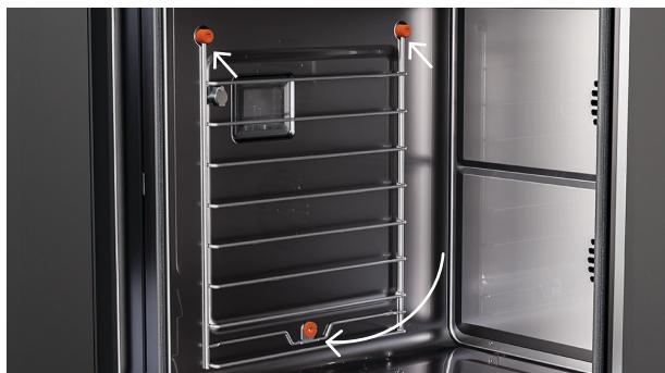
3. To replace, fit the top of the rack into the studs, then push the base of the rack flush against the side of the oven.
