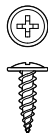
#8x16 mush washer screw (35x) (for Side trim attachment: Fixed screw method only (12x))
