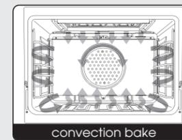
The heated air is circulated by the motorized fan in the rear of the oven providing a more even heat distribution. This even circulation of air equalizes the temperature throughout the oven cavity and eliminates the hot and cold spots found in conventional ovens. A major benefit of convection baking is the ability to prepare food in quantity using multiple racks—a feature not possible in a standard oven.
