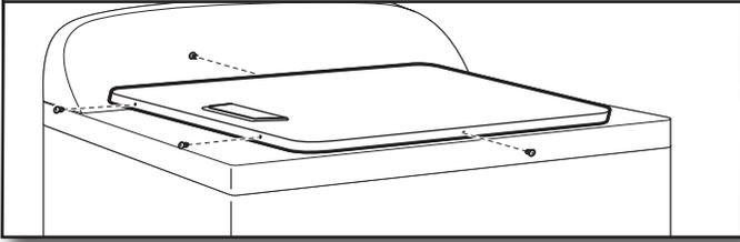
Remove screws at top, bottom, and side of door (4 screws) that hold the inner and outer door together. Holding door over towel on dryer, grasp sides of outer door and lift to separate it from inner door. Set outer door aside.
