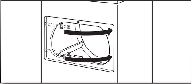
Remove the 4 screws that attach 2 plugs on the left side. Transfer plugs to opposite side using the same 4 screws.
