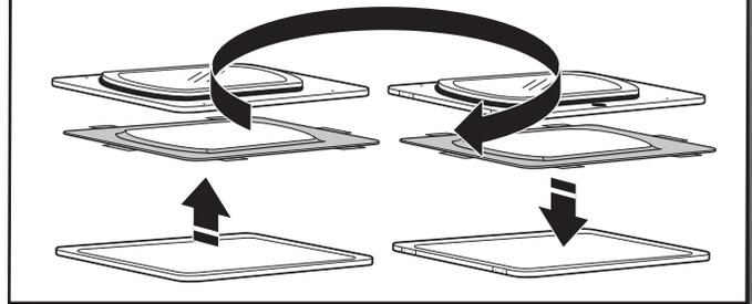
Rotate outer door 180° and set it back down on inner door. Be certain to keep cardboard spacer centered between doors. Reattach outer door panel to inner door panel so handle is on the side where hinges were just removed. Insert 4 door screws.
