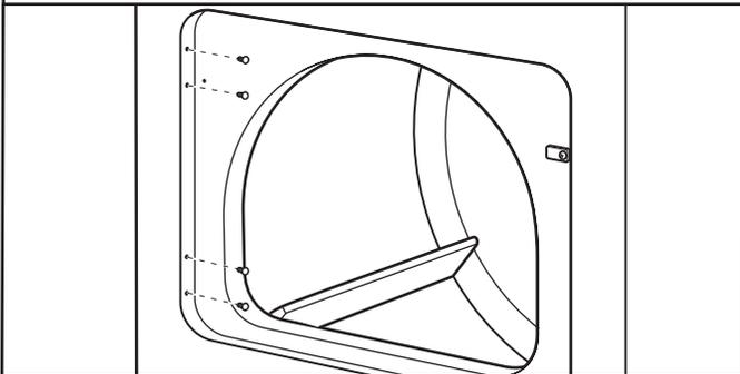
Use a small, flat-blade screwdriver to gently remove 4 hinge hole plugs on left side of dryer cabinet. Transfer plugs into hinge holes on opposite side of dryer cabinet.
