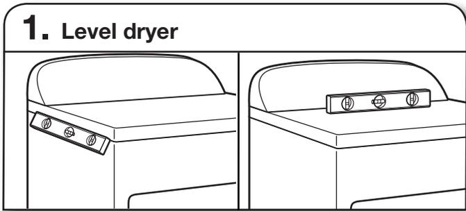
Check levelness of dryer from side to side. Repeat from front to back.
