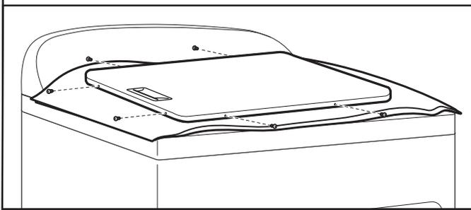
Remove screws at top, bottom, and side of door (6 screws). Keep door screws separate from hinge screws as they are different sizes. Holding door over towel on dryer, grasp sides of outer door and lift to separate it from inner door.
