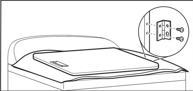
Remove screws attaching hinges to door.
