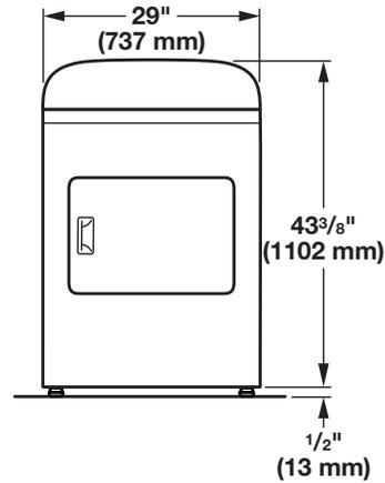
**NOTE:** Leveling legs should be 1/2" (13 mm) (to match height of 3.6 cu. ft. capacity washer) or 1½" (38 mm) (to match height of 3.8 cu. ft. capacity washer).
