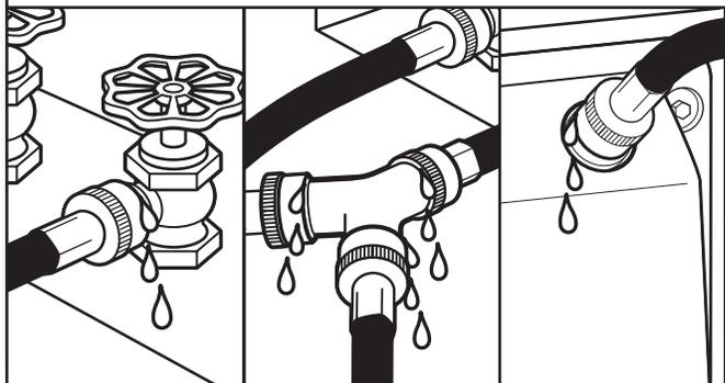
Check for leaks around "Y" connector, faucet, and hoses.
