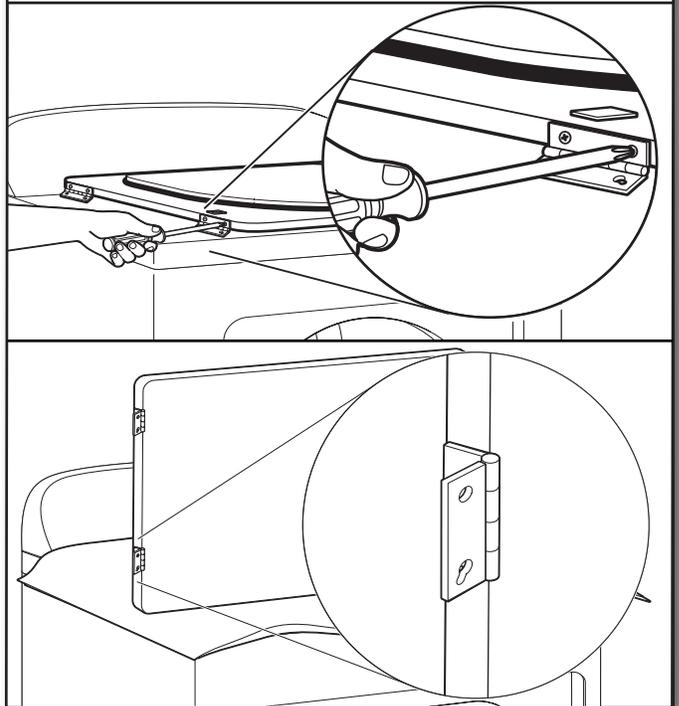
Reattach door hinges to dryer door so that the larger hole is at the bottom of the hinge.
