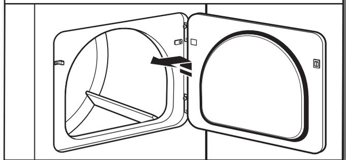
Lift door until top screws in dryer cabinet are in large part of hinge slot. Pull door forward off screws. Set door (handle side up) on top of dryer. Remove top screws from dryer cabinet.
