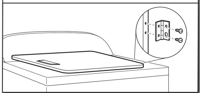
Remove screws attaching hinges to door.
