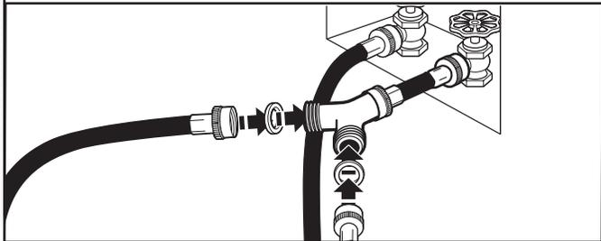
Attach dryer 5 ft (1.5 m) inlet hose ends to the "Y" connector. Attach washer cold inlet hose to other side of "Y" connector. Screw on coupling by hand until it is seated on connector. Using pliers, tighten the couplings an additional two-thirds turn.
