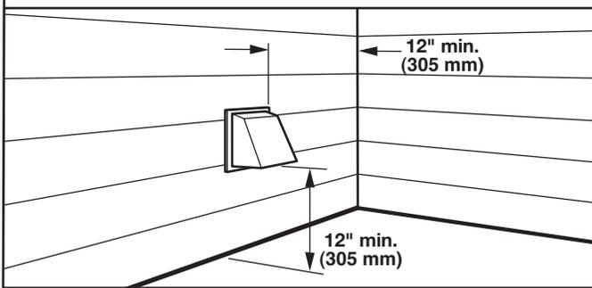
Install exhaust hood and use caulking compound to seal exterior wall opening around exhaust hood.
