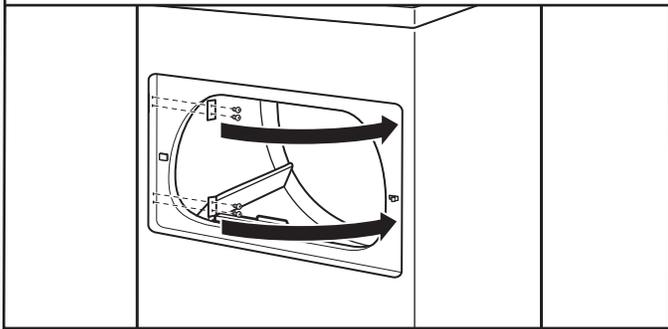
Remove the 4 screws that attach 2 plugs on the left side. Transfer plugs to opposite side using the same 4 screws.
