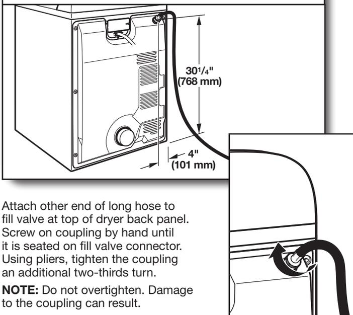
Attach other end of long hose to fill valve at top of dryer back panel. Screw on coupling by hand until it is seated on fill valve connector. Using pliers, tighten the coupling an additional two-thirds turn.
