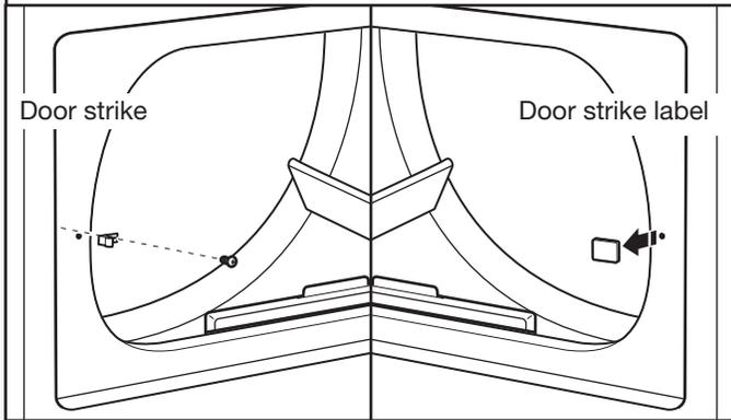
Remove door strike and door strike label from dryer cabinet. Insert the door strike into hole where door strike label was removed and secure with screw. Cover original door strike hole with door strike label and press firmly into place.
