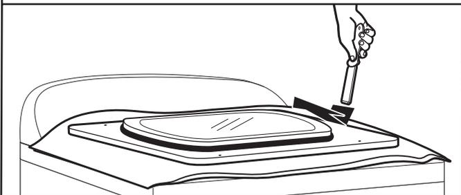
Holding door over towel on dryer, pry inner door and lift to separate it from outer door.
