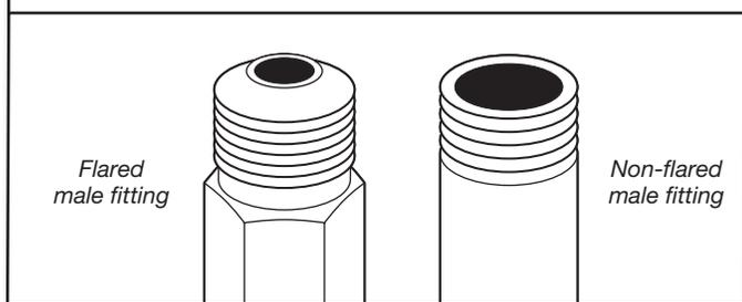
Remove red cap from gas pipe. Using a wrench to tighten, connect gas supply to dryer. Use pipe-joint compound on threads of all non-flared male fittings. If flexible metal tubing is used, be sure there are no kinks.
