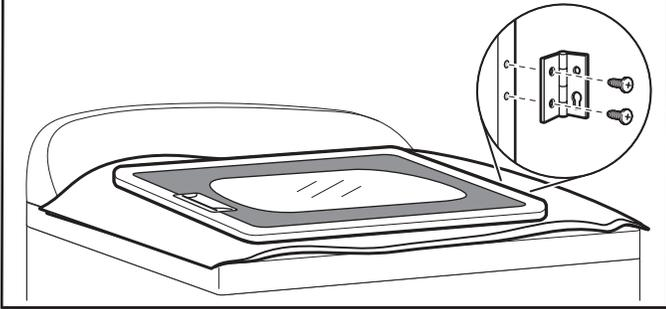
Remove screws attaching hinges to door.
