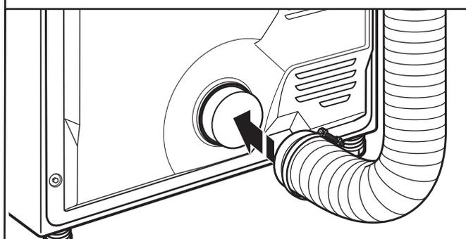
Using a 4" (102 mm) clamp, connect vent to exhaust outlet in dryer. If connecting to existing vent, make sure vent is clean. Dryer vent must fit over dryer exhaust outlet and inside exhaust hood. Check that vent is secured to exhaust hood with a 4" (102 mm) clamp.
