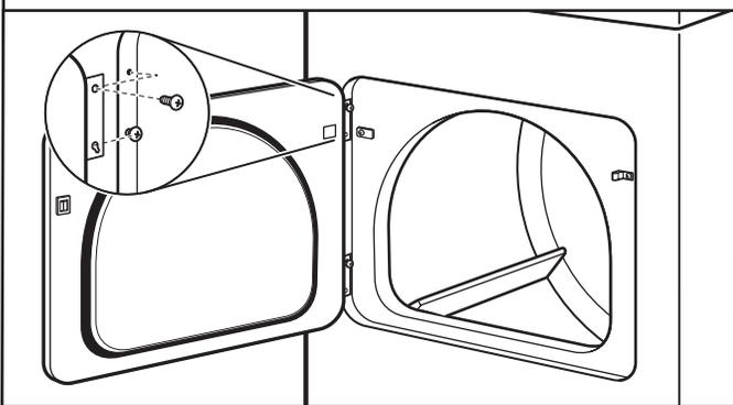
**NOTE:** Two people may be needed to reinstall door. Insert screws into the bottom holes on left side of dryer cabinet. Tighten screws halfway. Position door so large end of door hinge slot is over screws. Slide door up so screws are in bottom of slots. Tighten screws. Insert and tighten top screws in hinges.
