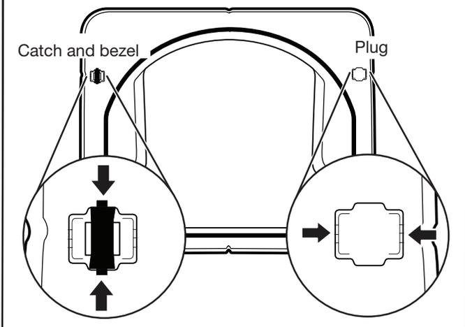
Remove the door catch, bezel, and plug from the inside of the inner door by squeezing and pulling/pushing them. Place the door catch, bezel, and plug on the sides opposite from where they were.
