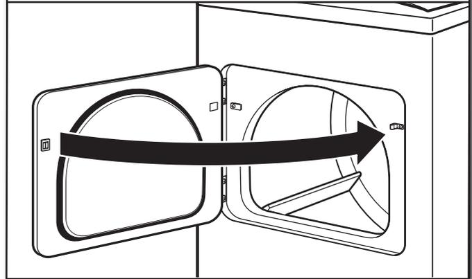
Close door and check that door strike aligns with door catch. If it is needed, slide door catch left or right within slot to adjust alignment.
