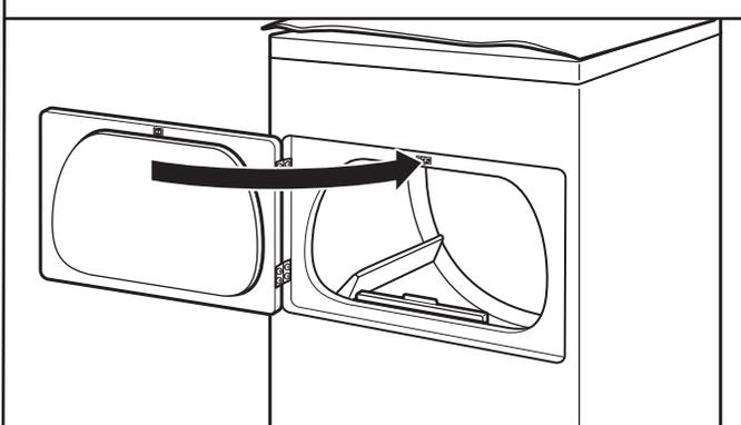
Close door and check that door strike aligns with door catch. If it is needed, slide door catch left or right within slot to adjust alignment.
