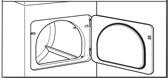
Open dryer door. Remove bottom screws from dryer cabinet side of hinges. Loosen (do not remove) top screws from dryer cabinet side of hinges.
