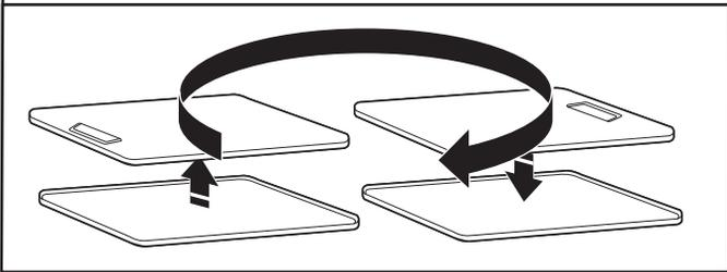
Rotate outer door 180° and set it back down on inner door. Reattach outer door panel to inner door panel so handle is on the side where hinges were just removed. Insert 4 door screws.
