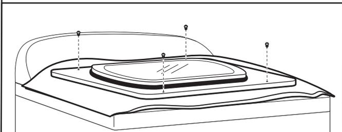
Remove screws at top, bottom, and side of door (4 screws). Keep door screws separate from hinge screws as they are different sizes.
