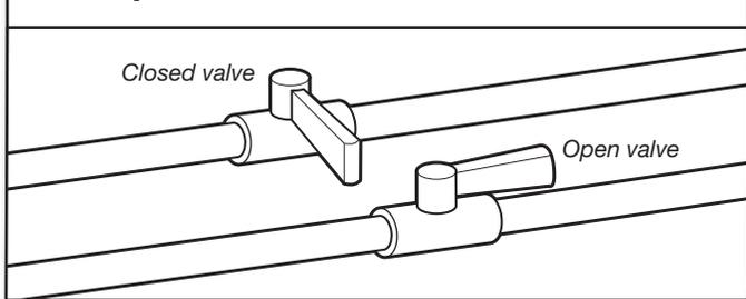
Open shut-off valve in supply line; valve is open when handle is parallel to gas pipe. Then, test all connections by brushing on an approved noncorrosive leak-detection solution. Bubbles will show a leak. Correct any leaks found.
