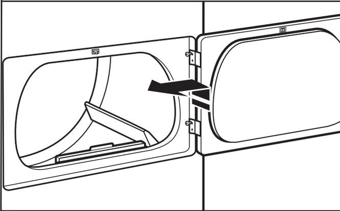
Lift door until top screws in dryer cabinet are in large part of hinge slot. Pull door forward off screws. Set door (handle side up) on top of dryer. Remove top screws from dryer cabinet.
