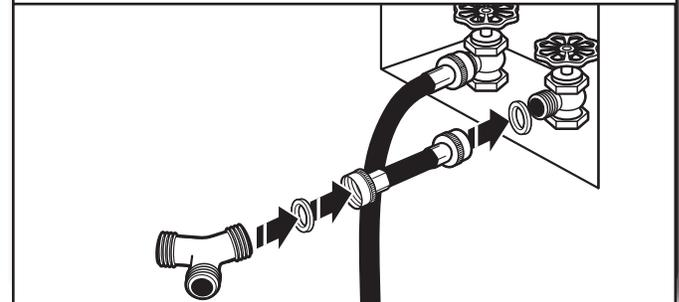
Attach 2 ft (0.6 m) inlet hose to cold water faucet. Screw on coupling by hand until it is seated on faucet. Then attach "Y" connector to end of the 2 ft (0.6 m) inlet hose. Screw on coupling by hand until it is seated on "Y" connector.
