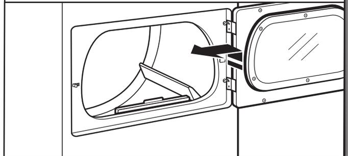
Lift door until top screws in dryer cabinet are in large part of hinge slot. Pull door forward off screws. Set door (handle side up) on top of dryer. Remove top screws from dryer cabinet.
