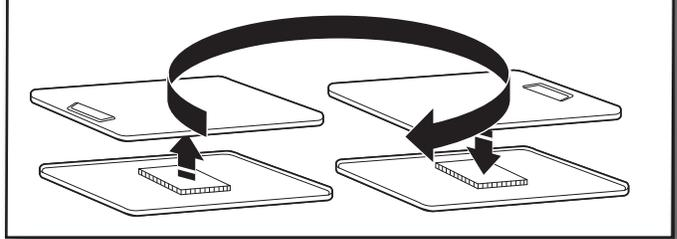
Rotate outer door 180° and set it back down on inner door. Be certain to keep cardboard spacer centered between doors. Reattach outer door panel to inner door panel so handle is on the side where hinges were just removed. Insert 6 door screws.
