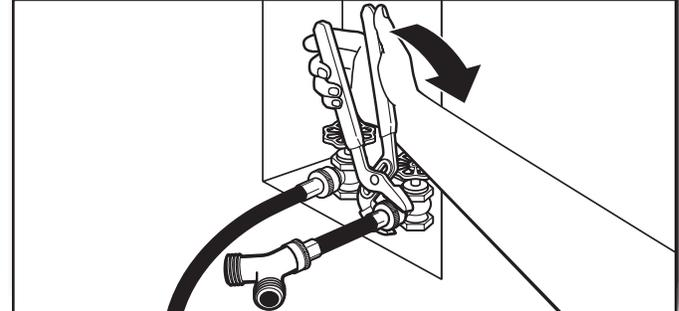
Using pliers, tighten the couplings with additional two-thirds turn.
