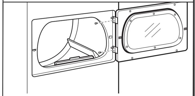
Open dryer door. Remove bottom screws from dryer cabinet side of hinges. Loosen (do not remove) top screws from dryer cabinet side of hinges.
