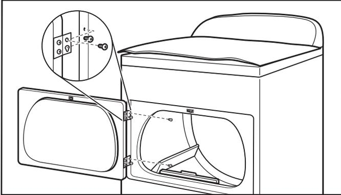
**NOTE:** 2 people may be needed to reinstall door. Insert screws into the bottom holes on left side of dryer cabinet. Tighten screws halfway. Position door so large end of door hinge slot is over screws. Slide door up so screws are in bottom of slots. Tighten screws. Insert and tighten top screws in hinges.
