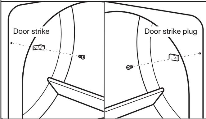
Remove door strike and door strike plug from dryer cabinet. Insert the door strike into door strike plug hole and secure with screw. Insert door strike plug into original door strike hole and secure with screw.
