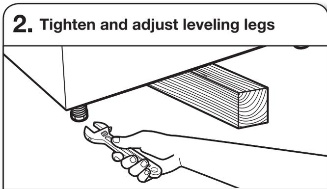
If dryer is not level or the same height as the washer, prop up using a wood block. Use wrench to adjust legs up or down, and check again for levelness. Once legs are level, make sure all four legs are snug against the floor before tightening them.
