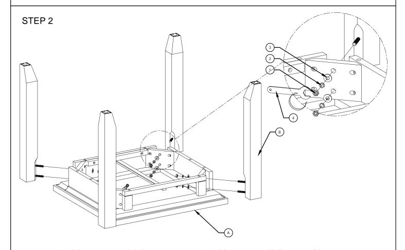
Step 2: Attach leg(B) into the top table(A). insert the hexagonal nut(1), lock washer (2), flat washer (3) into bolt, tighten with wrench(4).
