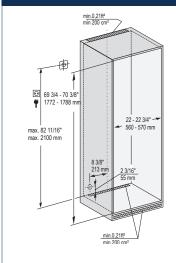
This is a fully integrated refrigerator appliance designed to be completely enclosed in a dedicated kitchen cabinet. This dedicated cabinet box must be constructed in accordance with the specified dimensions and must allow for sufficient air circulation to ensure proper operation. For more details about ventilation requirements, please refer to Design Guide.
