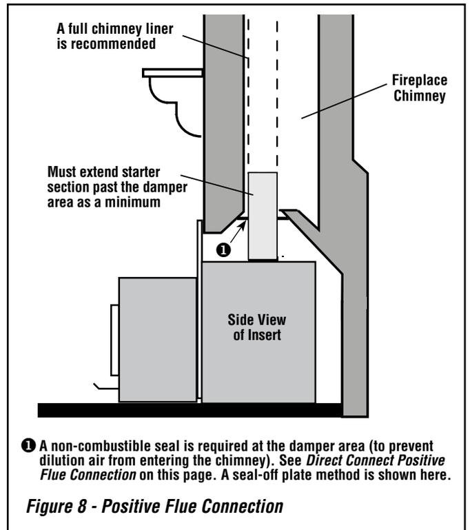
Figure 8 - Positive Flue Connection
