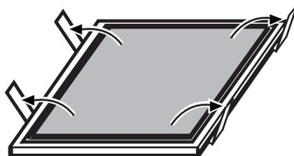
3. Place charcoal filter into top side of metal filter.
