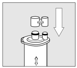
■ Remove the descaling cartridge and seal it with the cap.
