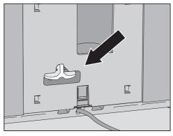
Insert the adapter in place of the descaling cartridge.
