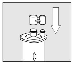
■ Seal the descaling cartridge with the cap.
