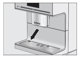
Remove the protective film from the drip tray cover and place it into the lower panel.
