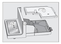
■ Remove the drip tray cover ①, the drip tray ②, and the lower panel ③.
