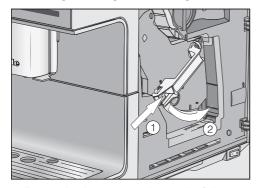
■ Press the button on the end of the handle of the brew unit ① and while doing so turn the handle clockwise ②.
