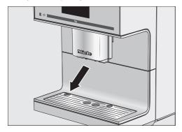
■ Reinstall the drip tray cover. Make sure that the drip tray cover is correctly installed (see illustration).
