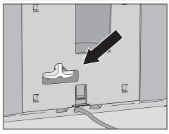
Insert the adapter in place of the cartridge. When the display goes out, the machine has finished evaporating.
