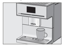
Place the cup under the hot water spout. ■ Select the type of tea on the display.
