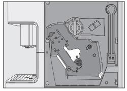
Clean the interior of the coffee machine. Make sure that the areas highlighted in the illustration are cleaned especially well.
