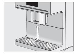
The central spout and cup rim sensor cannot be manually adjusted.
