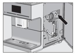
Push the slide control a maximum of one setting to the left (for finer grinding) or to the right (for coarser grinding).
