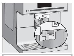
Push the cleaning brush a maximum of 3/4" (1 cm) into the steam jet.
