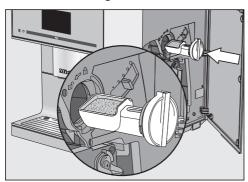
Fill the coffee scoop with ready ground coffee. Push the ground coffee drawer horizontally into the ground coffee chute. In order to not overfill the brew unit, place a maximum of **2** level scoops of coffee in the ground coffee chute.
