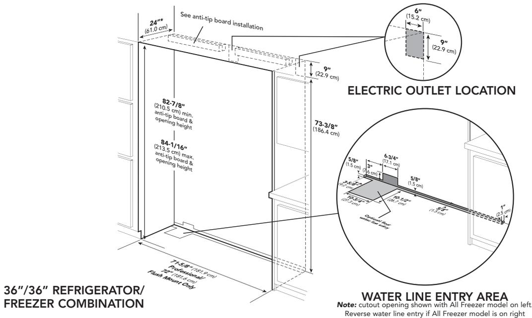
\*Custom panel models fit flush in 25"-deep (63.5 cm) cabinet openings. They can be installed in standard 24"-deep openings. The door faces and top grille will protrude 3/4" (1.9 cm) into the room.
