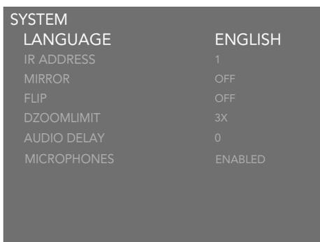
4. When an option is selected, press the < or > buttons to decrease or increase the value, respectively. If the option has an ON, OFF, or other string value, the same buttons can be used to switch between each value.
