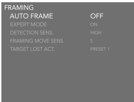
4. When an option is selected, press the < or > buttons to decrease or increase the value, respectively. If the option has an ON, OFF, or other string value, the same buttons can be used to switch between each value.
