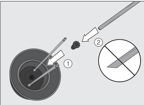
Make sure that you do **not** insert the slanted end of the stainless steel tube into the seal. This will damage the seal.
