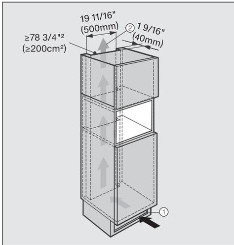
– Air intake ① occurs via the plinth at the bottom of the appliance and the air escapes at the top ② at the rear of the surrounding cabinets.
