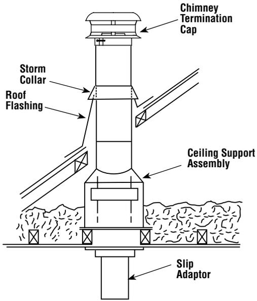
Single wall stove pipe must not pass through attics, closets, walls or ceilings. It is used to connect this appliance to a factory built or masonry chimney.
