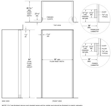
NOTE: 31/2" (89) finished returns and shaded areas will be visible and should be finished to match cabinetry Shaded line represents profile of unit brit/a" (19) panel.
