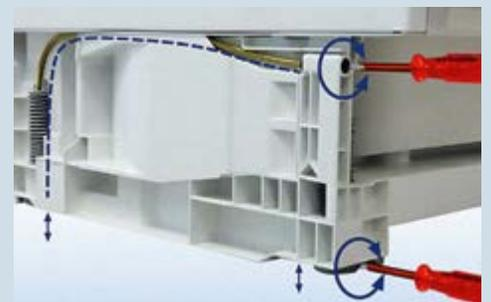
**Vario Toe Kick:** The Vario Toe Kick permits the adjustment of kitchen units in height and depth. All four height-adjustable feet permit adjustment from the front within a 2" range. In addition, the ventilation grille can be adjusted within a range of 2" to match the front of the kitchen units.
