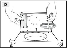
**Fig.3D:** Position the electrical box so it is in line with the holes of the previously removed screws and tighten.
