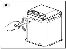
Fig.3A: Remove the central screw.
