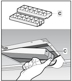
**Fig.9:** The charcoal fi lters **C** must be fitted in the ducting unit located inside the hood.
