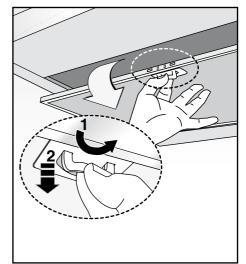
**Fig.8:** Remove the aluminum panels by pulling the lever **1** out and pushing downwards **2**.
