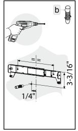
Fig.2: Make a mark on the wall and then drill a hole 1/4" inches away from the middle of the bracket. Insert the expansion plug.
