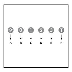
• By pressing key **F** for two seconds (with the hood switched off) the "**clean air**" function is activated. This function switches the appliance on for ten minutes every hour at the first speed. As soon as this function is activated the motor starts up at the first speed for ten minutes, During this time key **F** and key **C** must flash at the same time.
