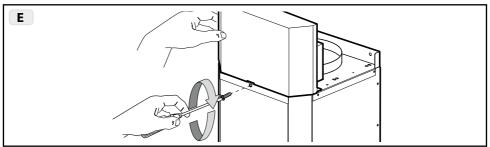
**Fig.3E:** Pay attention that the tear tape of the electrical box is inside the slot and then tighten screw.
