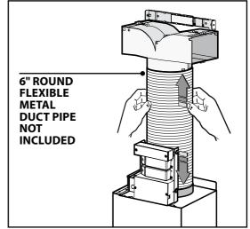
**Fig.6**: Once the air diverter has been inserted into the bracket and fastened to the wall connect the flexible (6" Round Metal) pipe to the diverter, use duct tape to seal
