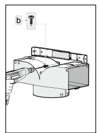
**Fig.5:** Fasten the air diverter permanently to the wall with a screw (the hole previously drilled in **Fig.2**).
