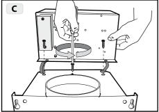
Fig.3C: Remove the 3 fixed screws.
