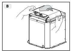
Fig.3B: Lift the electrical plant box.
