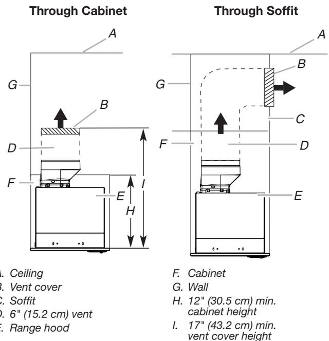
**NOTE:** 12" (30.5 cm) high cabinets without a soffit may allow the 6" (15.2 cm) vent and vent cover to be seen.
