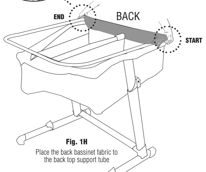
**4** Place the back bassinet fabric over the back rail tube. Align and fasten zipper to top rail (Fig. 1H).
