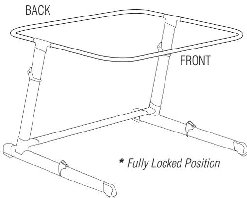
**3** Align top back support tube to the side frames. Insert both sides of the top support tube into the bassinet frame until holes are aligned (Fig. 1F). After top support is in place, insert nut & bolt as shown (Fig. 1G) and use the wrench to tighten screws in clockwise direction.
