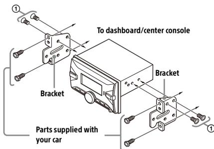
When mounting this unit to the preinstalled brackets of your car, use the mounting screws ① in the appropriate screw holes based on your car: T for TOYOTA and N for NISSAN.
