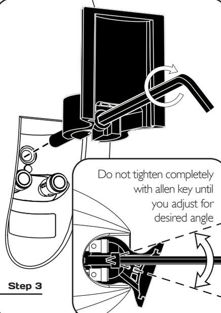
Do not tighten completely with allen key until you adjust for desired angle
