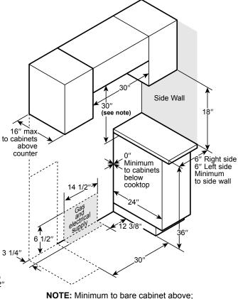
see Installation Instructions for alternate installation configurations.
