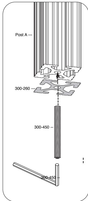
**B.** Screw the rear and side posts through the panel and into the bottom posts. Be sure to square the post with the shelf. Do not over tighten.
