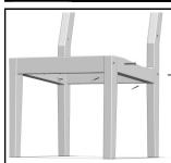
Align Front and Rear Aprons with Front and Rear Legs. Secure with (4) 50mm Hex Lags through
