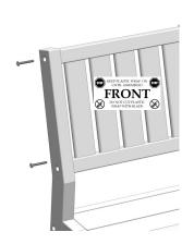
Secure Back Assembly to Side Assembly using (4) 50mm Lags. Note: Tag location describing "FRONT"
