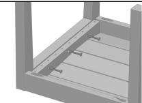
Secure Seat Assembly to Side Assembly using (6) 50mm LAGS.
