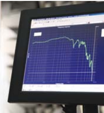
Testing the limits: a display shows the frequency response of a Nautilus drive unit. Nautilus tweeter domes rims are reinforced with carbon fibre, which raises the first break-up threshold by 30 per cent, pushing it up to twice the limit of human hearing.
