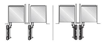
If there is a partition with a thickness from  ${}^5/_8$ " (16 mm) to 6  ${}^5/_{16}$ " (160 mm) between the adjacent appliances, then each appliance should be individually installed within its own niche using the mounting accessories included.
