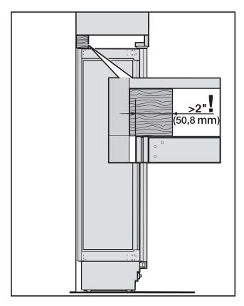
If the anti-tip brackets cannot be attached securely, an alternative anti-tip device can be used. Ensure that there is no "give" between the appliance and the anti-tip device.
