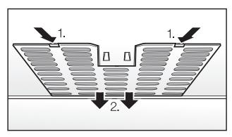
■ Unhook the filter cover, **1.** in each side of the drawer and remove them along with the filter mat downwards starting from **2**.
