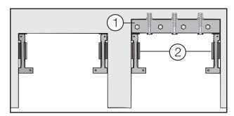
If the installation niche is deeper than the appliance, a solid wooden beam ① can be placed behind the anti-tip brackets ② so the appliance can be securely attached to the base or wall.
