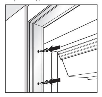
■ Fasten the appliance on the left and right hand sides with the 3 (supplied) wood screws.
