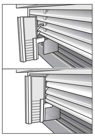
■ Clip the air separator, left and right of the partition, in the exhaust grille. Be sure that it clicks into place and guides the foam partition under the exhaust grille.
