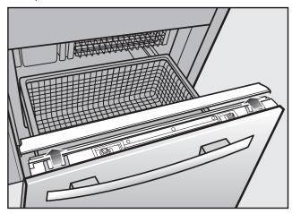
■ To remove the stainless steel front, loosen the two nuts and remove the cover strip.
