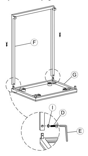
Step 5: Do not fully tighten the bolts
