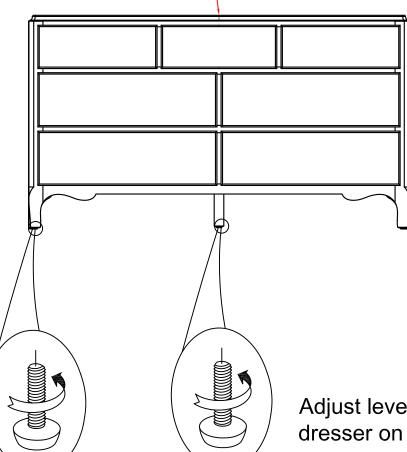
Adjust leveler if needed to level dresser on uneven floor.
