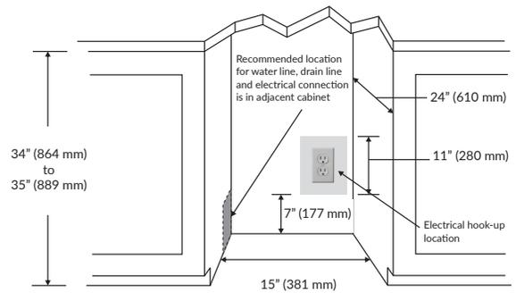
NOTE: For Gravity drain models, the drain hole cannot exceed 7 inches above the floor.
