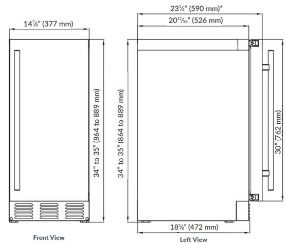
\*Dimensions are the same for Panel Ready unit when ¾" panel applied
