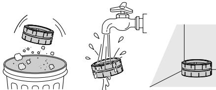
**7** Assemble a completely dry exhaust filter ❶ to the product.
