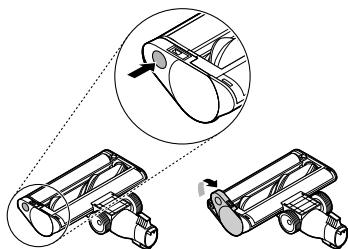
**6** Use a damp towel or cloth to remove any remaining foreign objects and dust from both the brush and the bottom of the nozzle.
