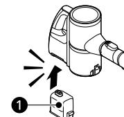
**2** Attach the nozzles, tools, or Fixed pipe by sliding them onto the inlet **2** on the body until they click into place. The nozzles and tools can also be attached to the end of the Fixed pipe **2**.
