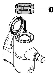
**8** Close the exhaust filter cover, press down and turn it to the right to lock the cover.
