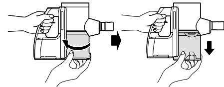
**7** Remove dust from the dust bin, Cyclonic Mesh Filter, and pre-filter using a cleaning brush, etc., and wash them with water at least once a month.
