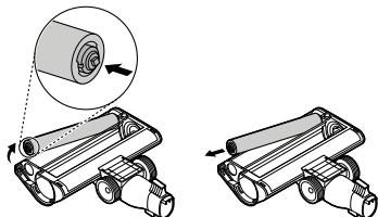
**7** Slide the brushes back into the nozzle and rotate the cover back into place. Turn the cover lock clockwise to lock the cover.
