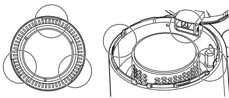
**6** Clean the exhaust filter by brushing the dust off it regularly and wash it in running water at least once a month.
