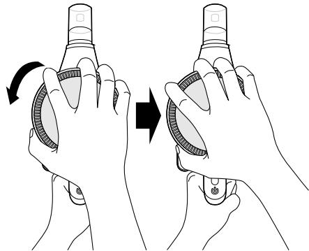
**9** Turn the product body over again and shake it while pressing down the lever to remove the dust.
