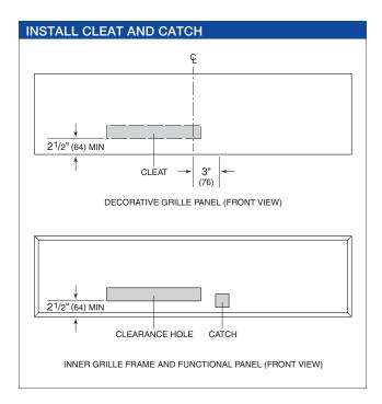
The cleat must be located to the left of a line 3" (76) to the right of the center of the built-in unit, to clear the system fan shroud.
