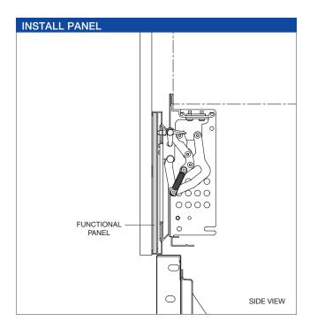
A ¹/4" (6) thick functional panel must be installed in the inner grille frame (the part that flips up) to prevent warm air discharge from short-circuiting back into the system.
