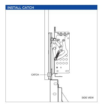
Depending on the design and size of the catch, it will need to be recessed into the functional grille panel and maybe partially into the decorative grille panel.
