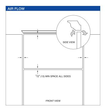
Allow for at least  $^{1}/_{2}$ " (13) space on all four sides of the grille panel for proper air flow to the refrigeration system. For flush inset models, this is around the sides, top and bottom of the decorative grille panel.
