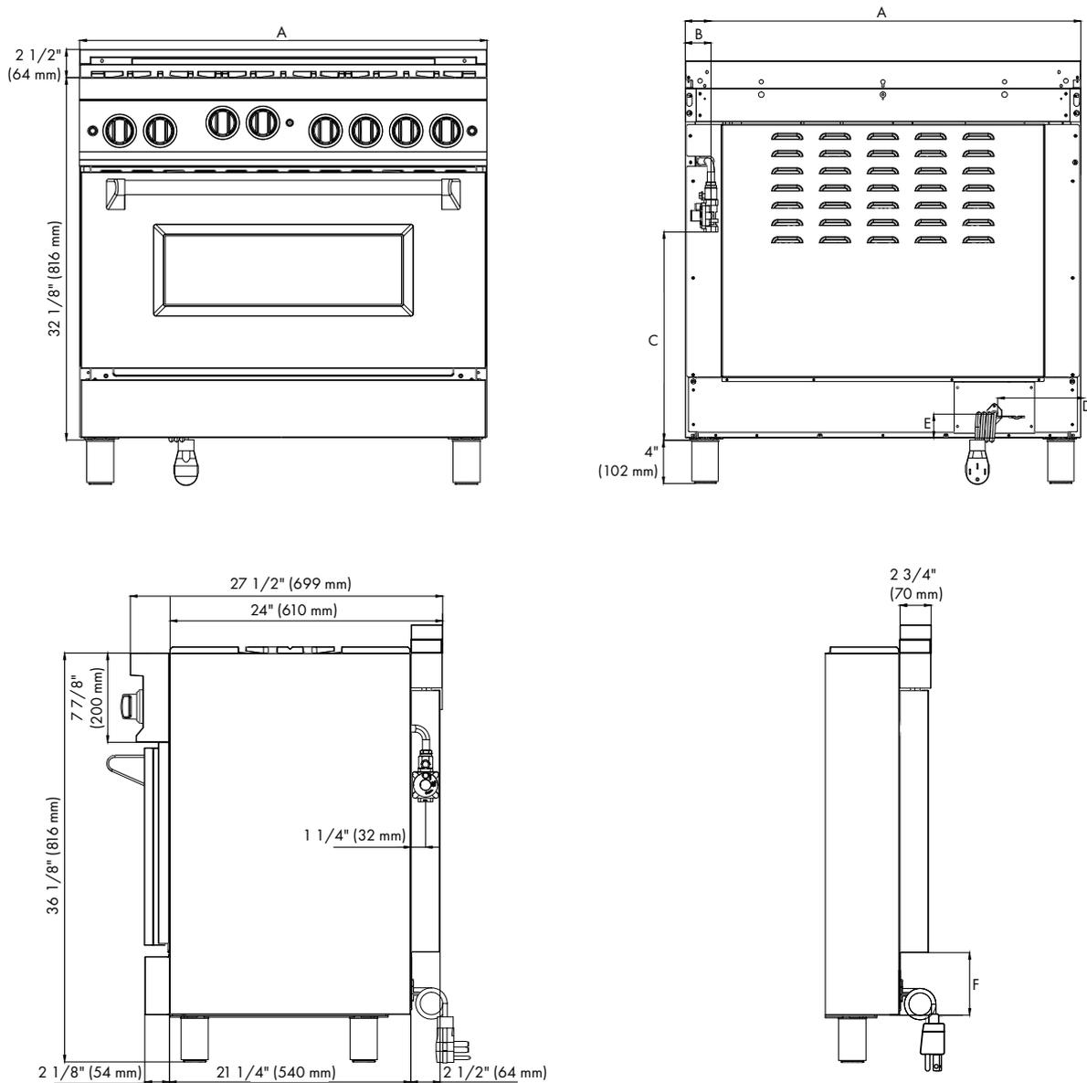
**NOTE:** The above diagram is of the RG36 series range; the measurements listed without a letter are universal across all RG models. See the next page for dimensions by model, and for in-depth product and cutout dimensions, see pages 10–11.
