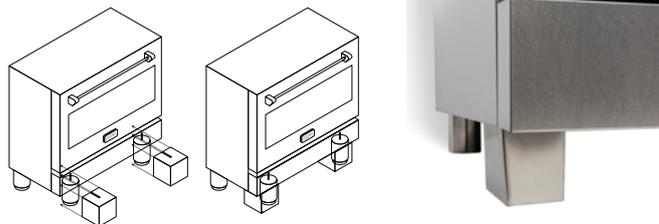
**NOTE:** If the range is not level, the cooking will be uneven. When adjusting the legs, ensure they are the same height.
