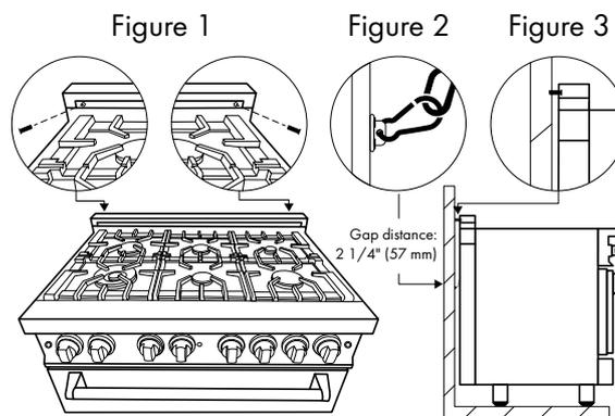
1. Measure the distance from the floor to where the chains connect on the back of the appliance.
