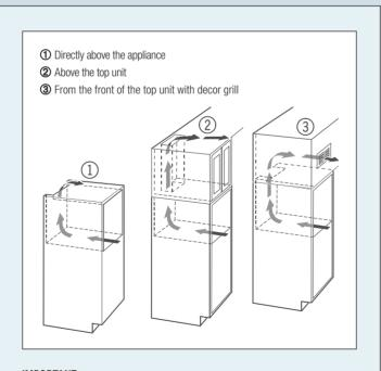
IMPORTANT When using decor grills, the sum of the individual openings must total a minimum of 31 square inches. A cut-out section of 31 square inches (200 cm<sup>2</sup>) for installing the ventilation grill is thus not sufficient.
