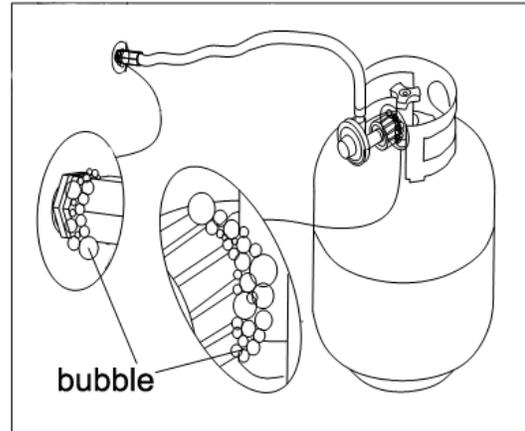
**NOTE:** When leak testing this appliance, make sure to test and tighten all loose connections, including the side burner. A slight leak in the system can result in a low flame, or a hazardous condition. gas tanks now come equipped with a leak detector mechanism internal to the tank; when gas is allowed to escape rapidly, it shuts off the gas supply. A leak may significantly reduce the gas flow making the side burner difficult to light or causing low flames.
